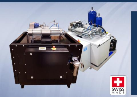
Our high-pressure pump produces the optimal pressure to clean your screens.
